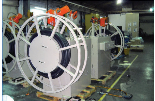
CABLE REEL WITH OPTICAL FIBRE FOR HIGH-VOLTAGE AND LOW-VOLTAGE
