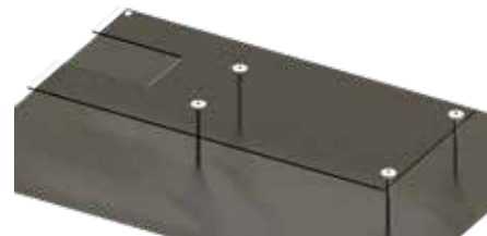
Contact protection with wing nuts and spacers
